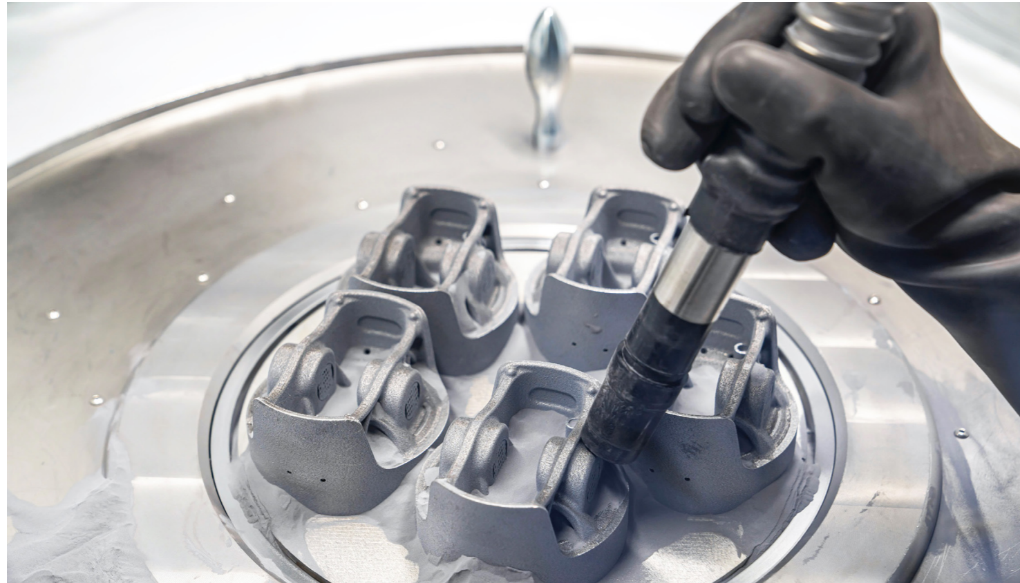
From a 3D printer: Innovative pistons for increased power and efficiency Image source: Porsche AG
